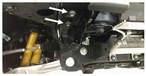
13. Remove the adaptive cruise control (ACC) sensor shroud from the vehicle using a panel pry tool to release the plastic clips. Using an 8mm socket wrench remove the ACC sensor with bracket from the intercooler. Figure 12.
