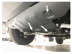
12. Using the 15mm socket wrench, remove the front bolt and loosen the rear bolt that attaches the skid plate mounting brackets to the frame letting the two brackets hang down.
